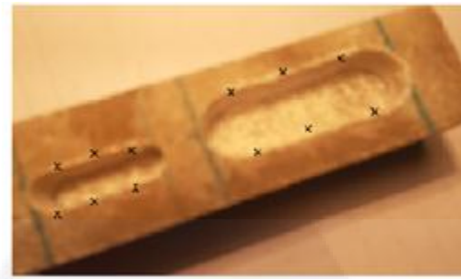
Fig. (1) Defects at groove walls surfaces.
